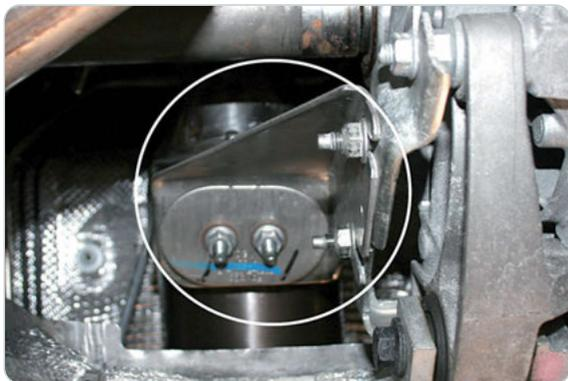
We recommend that you replace the clamps and the gaskets between the tuning catalyst and the turbocharger/engine and between the catalyst and the exhaust system.
